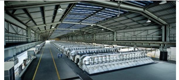
Smelting is the process of extracting Aluminium metal from alumina through electrolytic reduction
